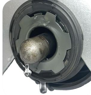
A few drops of water within the caliper can cause corrosion and lead to caliper failure.
