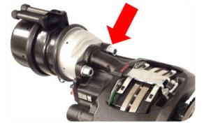
Tighten the air chamber's installation nuts in an alternating sequence so the chamber mates flush to the caliper.
