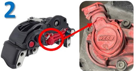
Examine the caliper's chain cover for cracks or damage and replace as required. Replace the caliper if water has caused rusting on the internal components.
