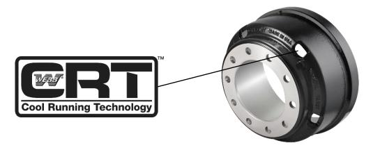
Webb's 66764 Trailer Drum features **Patented CRT (Cool Running Technology) vents**. This advanced design maximizes air flow into the wheel-end for superior heat transfer efficiency and cooler wheel-end operating temperatures. Cooler temperatures mean longer brake life and lower maintenance costs. Designed, cast, and machined in the **USA**.
