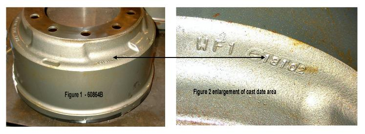
If the "Platinum Series" brake drum is not one of the cast date codes covered in this recall, then the vehicle can be returned to service after placing a blue dot (sticker) on the VIN number plate.
