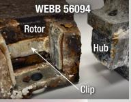
The patent-pending Webb design features a stainless steel clip that adds a protective barrier between the rotor and hub.
