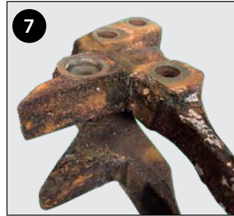
7 Check the general condition of the carrier and clean if required. Ensure the pads are sitting correctly in the carrier.
