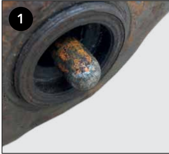
1 Check for signs of water damage on the air chamber pushrod.
