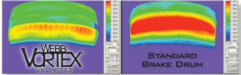
These photos taken from an infra-red camera mounted on the Webb Link dyno show a Webb Vortex<sup>®</sup> Unlimited drum next to a standard drum at precisely the same moment during braking. Compare the heat (red color) and you can actually see that Webb Vortex<sup>®</sup> Unlimited brake drums run significantly cooler.
